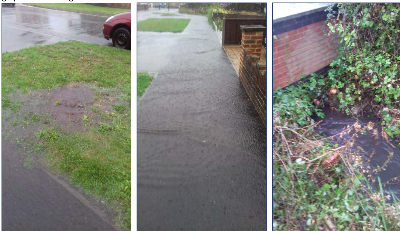
Photographs show manhole lifting on Fairlands Avenue and volume of water, together with water level in ditch.
