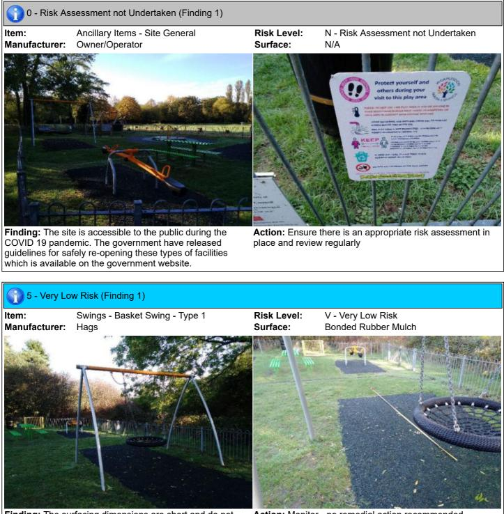
**Finding:** The surfacing dimensions are short and do not meet with the requirements of the current applicable standard
